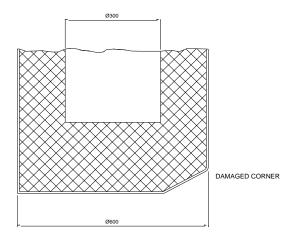
The damaged base may be turned off, back to an un-deformed area of the flask body.
