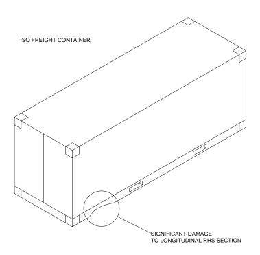
The area of damage was cut out, prepared for welding by removing all corrosion and paint in the area of the weld, a new piece fabricated, and then welded in place. The weld repair was approved by Lloyds Register, and subject to NDT post welding.
