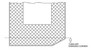
The lead should then be counter bored so that the area where weld is to be laid is not going to result in the lead melting and to ensure there is no lead contamination of the weld. Consideration should be given to profiling the lead surface to ensure keying of new lead. This would be particularly important if the lead was providing radial shielding.
