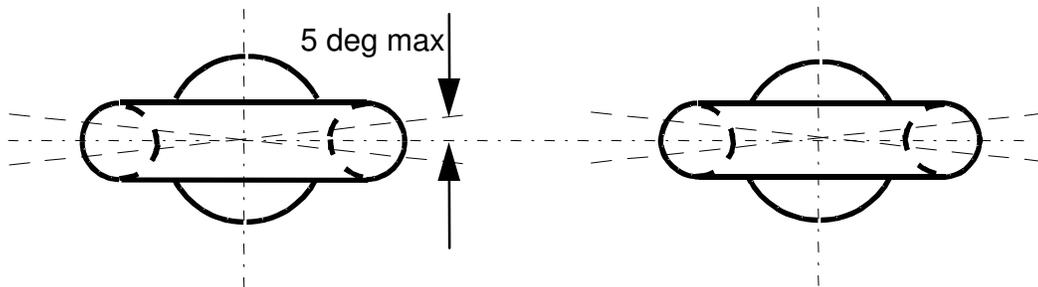
Figure 2 (b): Maximum misalignment of a pair of eyebolts
