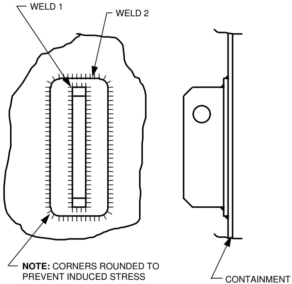
Area of Weld 1 is less than the area of Weld 2. Therefore Weld 1 will fail in preference, leaving the containment intact.
