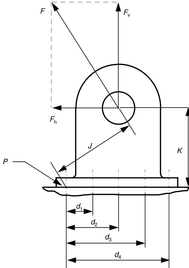
Figure A 3. Bolted lug, secured with 10 bolts
